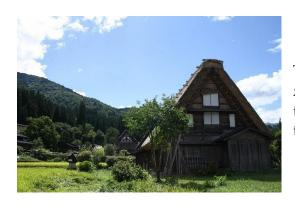
This style of farmhouse is called "gassho-zukuri" and is recognizable by the heavy thatched roofs that are designed to withstand the heavy snowfall of the cold winters.
